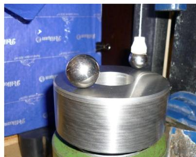
Fig. 8. Disc's deviation from horizontal plane test and contact point position identification
